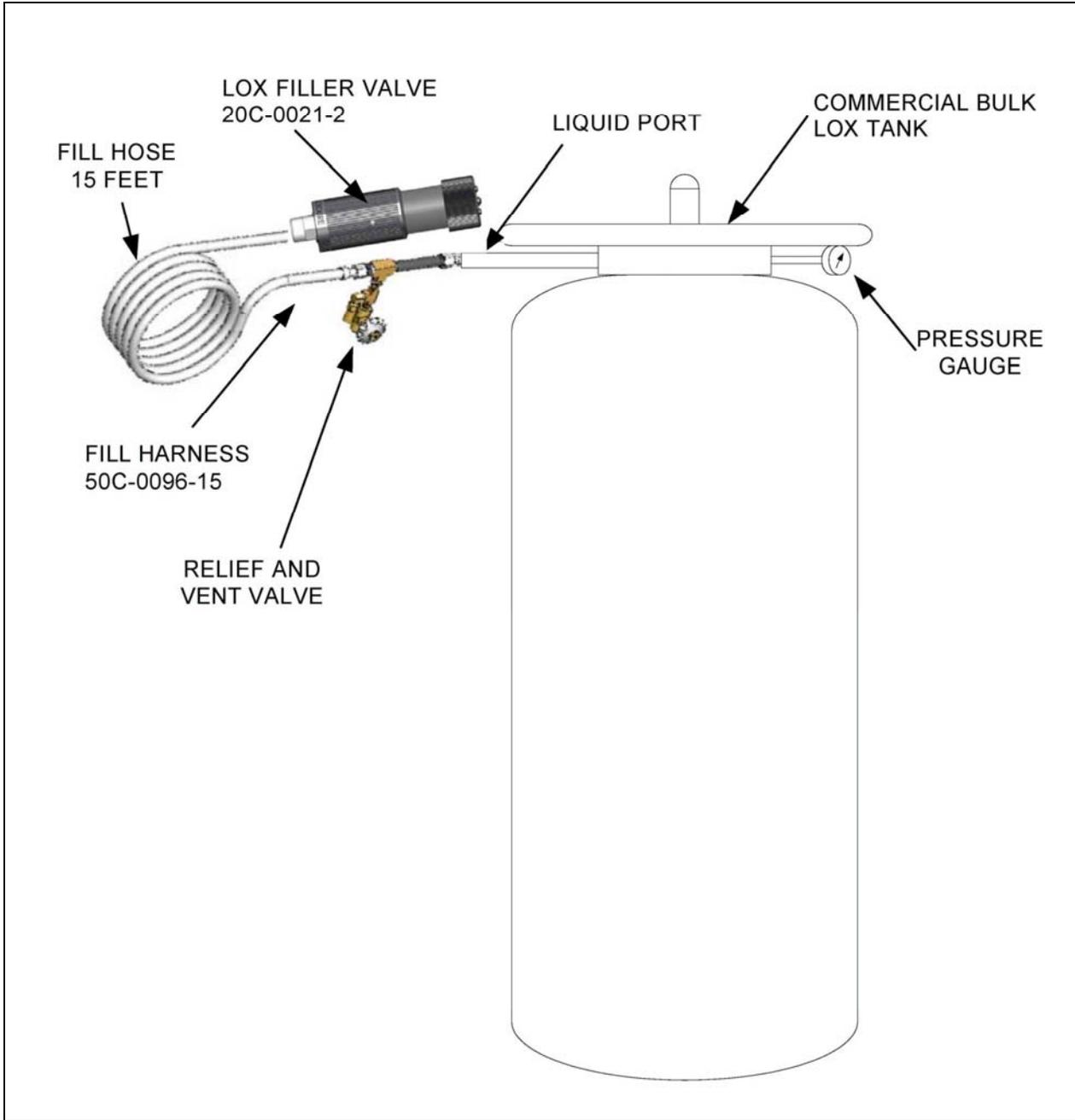
Figure 19 – Bulk LOX Storage Tank with Filling Harness
