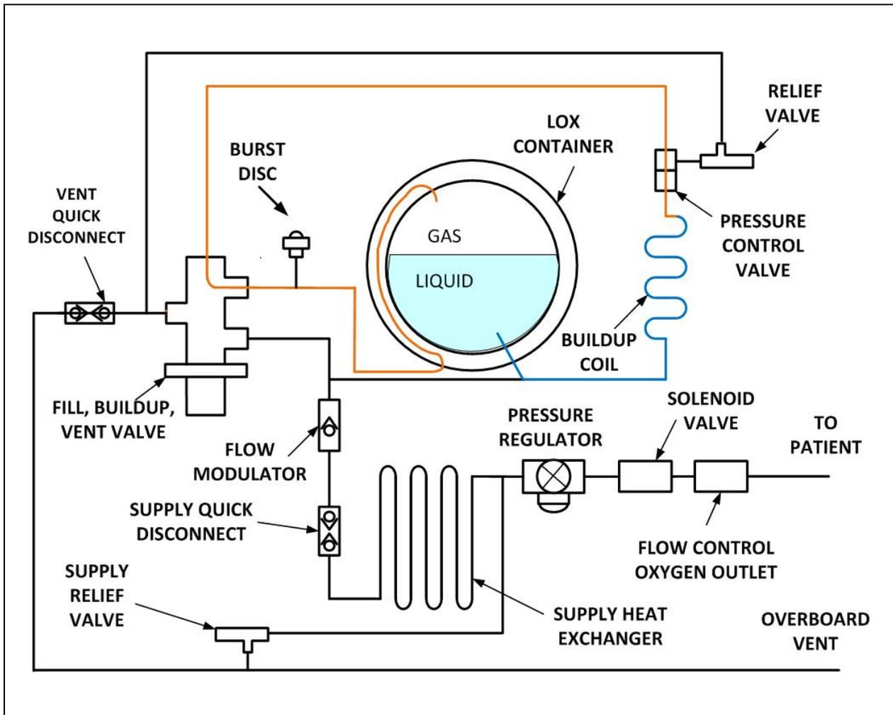
Figure 14 – Pressure Buildup Mode Schematic
