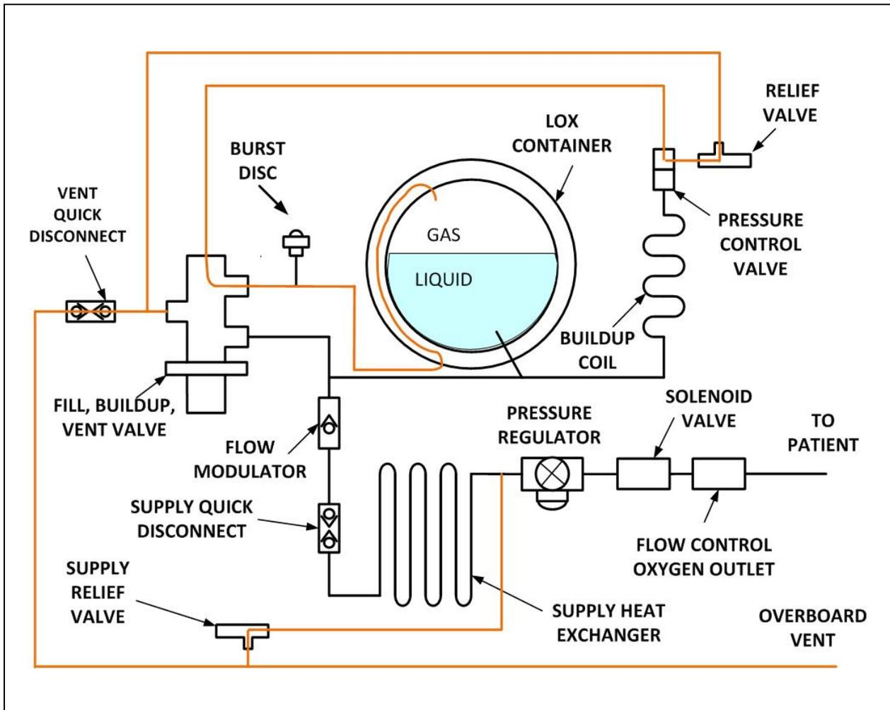
Figure 16 – Pressure Relief Mode Schematic
