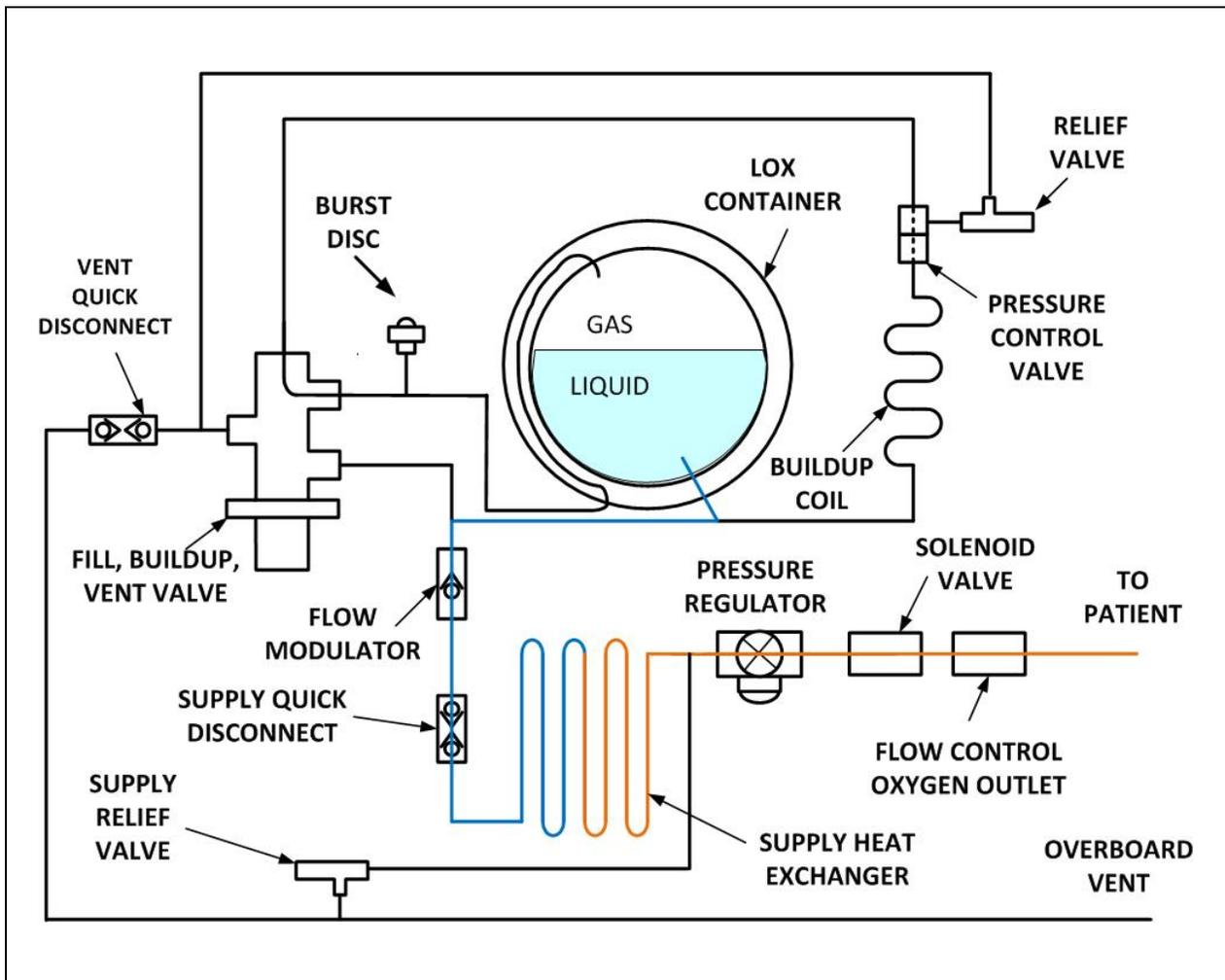
Figure 15 – Operating Mode Schematic
