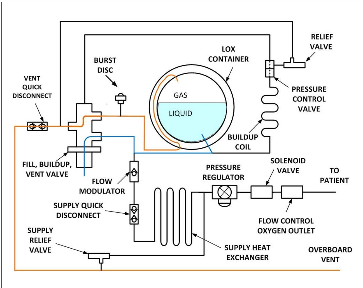
Figure 13 – Fill Mode Schematic
