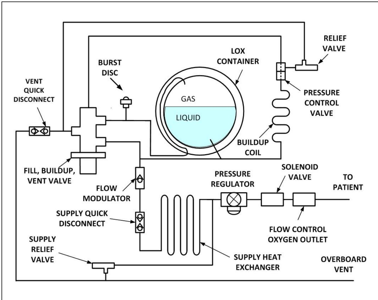
**Figure 12 – LOX System Schematic**
