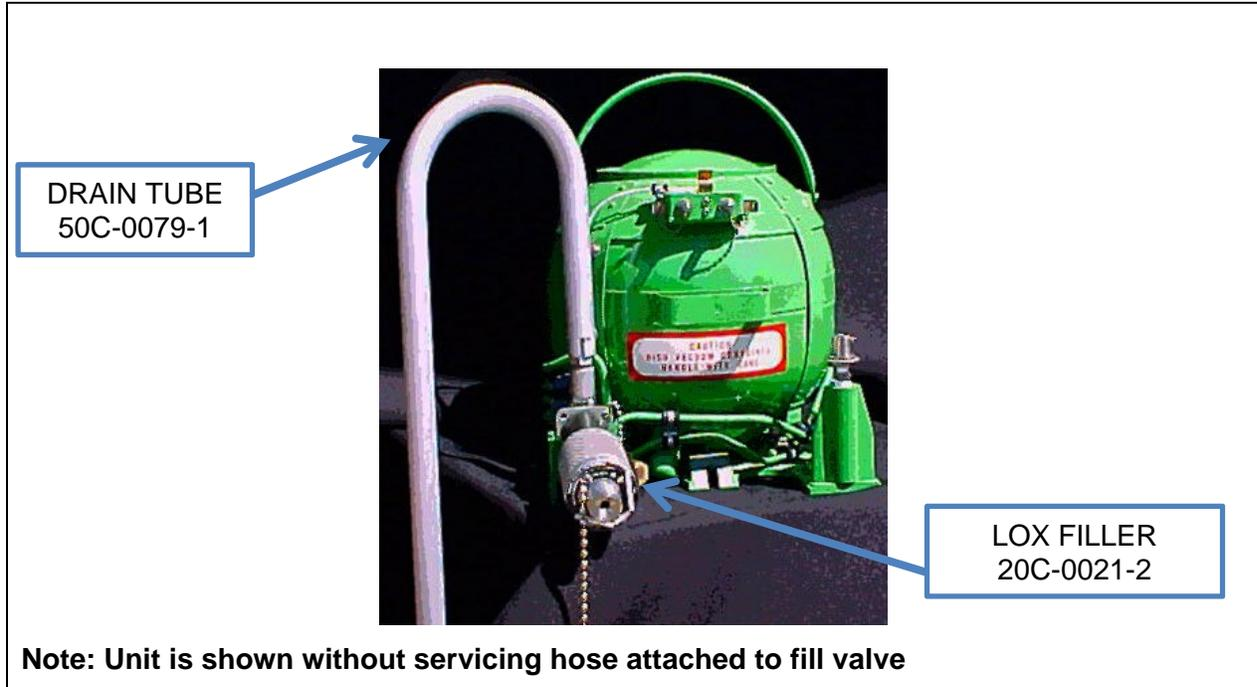
Figure 18 – LOX Servicing Connections
